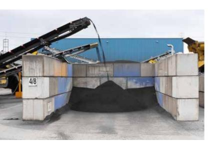
ALFA SINSTONE®, GRIPSTONE® and SICILYSTONE are by-products obtained from the recovery of black steel mill slag composed mainly of iron, calcium and silicon oxides, which is generated during the melting process of ferrous scrap in the electric arc furnace. These are high-performance artificial aggregates resulting from continuous research into new materials and new technologies for improving manufactured products and safeguarding natural resources.
