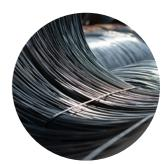
The products made by ribbed wire rods have a chemical composition in compliance with national regulation of destination countries where they are sent. On the other hand smooth wire rods have a specific composition based on the type of steel requested by the customer. The main materials of the final product are: iron >96%; alloy elements (e.g. manganese, silicon, carbon) 2% c.a.; other elements (e.g. copper, nickel, chromium), complementary to 100%.
